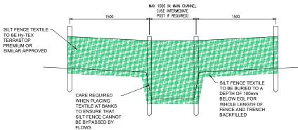
ELEVATION ON SILT FENCE AT DRAINAGE CHANNEL
